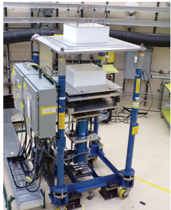
Planet loaded with CWS critical assembly. Note the configuration is split into two pieces to keep the assembly from becoming critical while workers are in the room. The lower platen is raised remotely to lock in with the stationary upper stack to achieve criticality (see Figs. 5 and 6 on previous spread).
