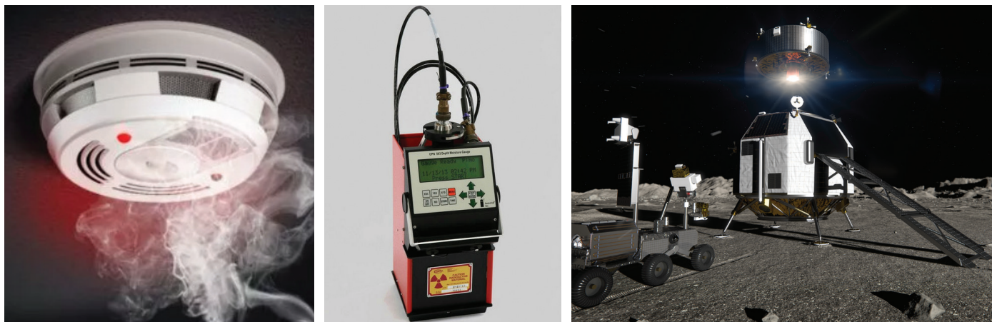
Figure 5. Americium-241 finds applications in smoke detectors ( left ), neutron moisture meters ( center ), and radioisotope thermoelectric generators (RTGs) for space exploration. Right: Artist's impression of a European Space Agency (ESA) Argonaut mission on the Moon. These missions, scheduled for launch in the 2030s, will use an americium-241-powered RTG to eliminate the need for solar panels and allow exploration of regions with little or intermittent sunlight.
