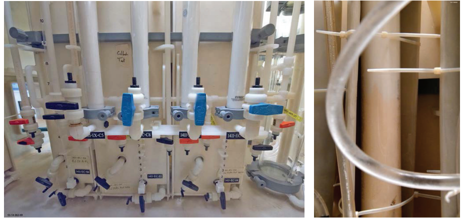
Figure 9. Column chromatography line in CLEAR process, used to extract americium-241 from a waste product stream in the EXCEL process.
